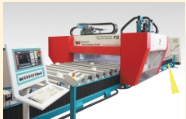
Safety shock absorbers attached to the moveable part of the production line
